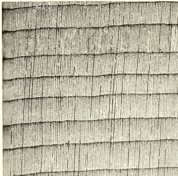
FIGURE 2-29.—Port Orford white-cedar. Cross section magnified 15 diameters.
